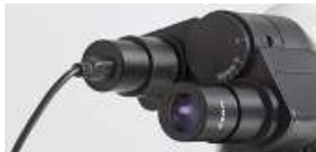
Eyepiece camera fixed into the tube
