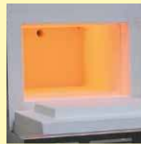
Muffle heated from four sides
