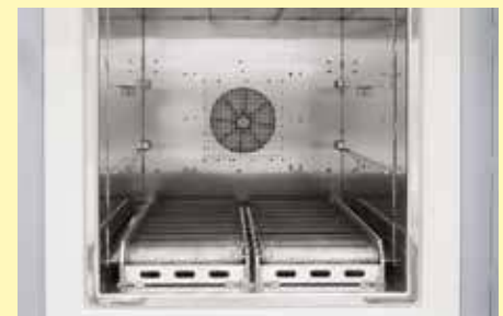
Roller conveyor in furnace chamber
