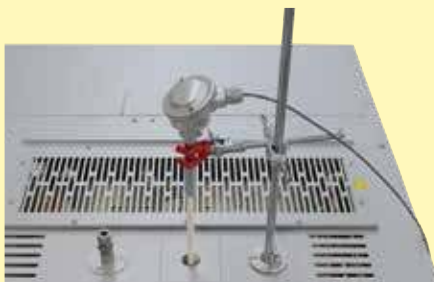
Thermocouple port in the ceiling with tripod
