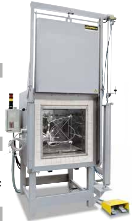
Holding frame for measurement of temperature uniformity
