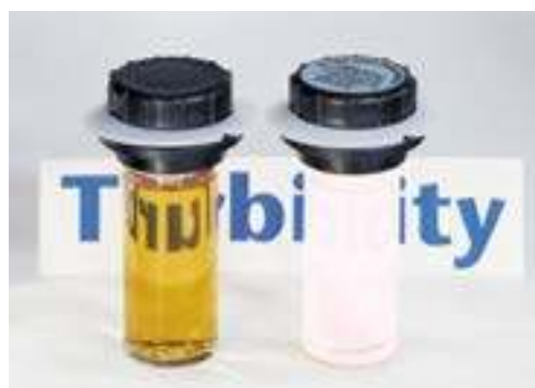
Turbidity measuring cuvette and standard cuvette
